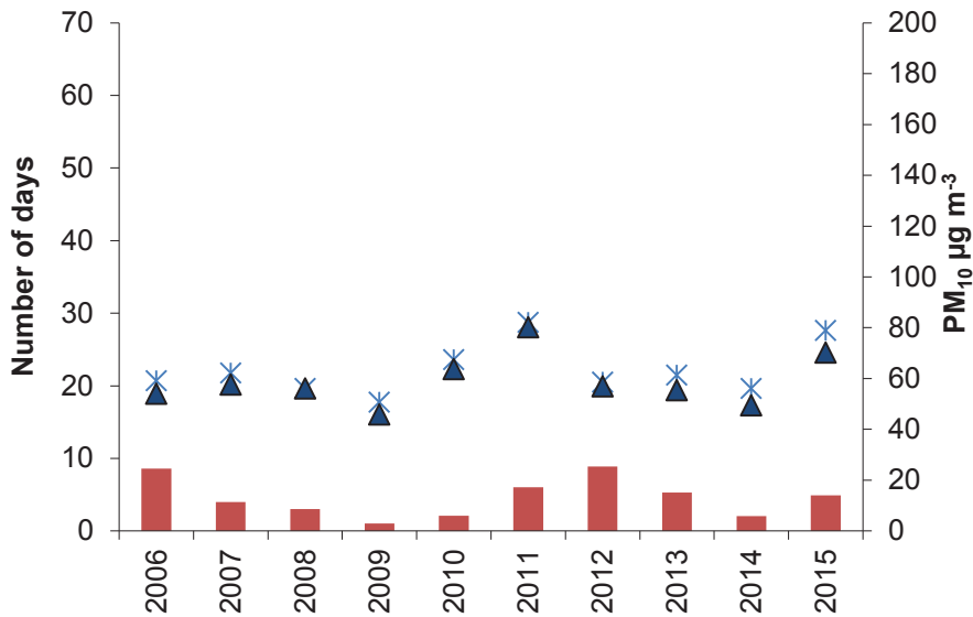
Figure 3.10: Number of days when 50 \mu\text{g m}^{-3} was exceeded, the maximum concentration and the second highest concentration from 2006 to 2015.
