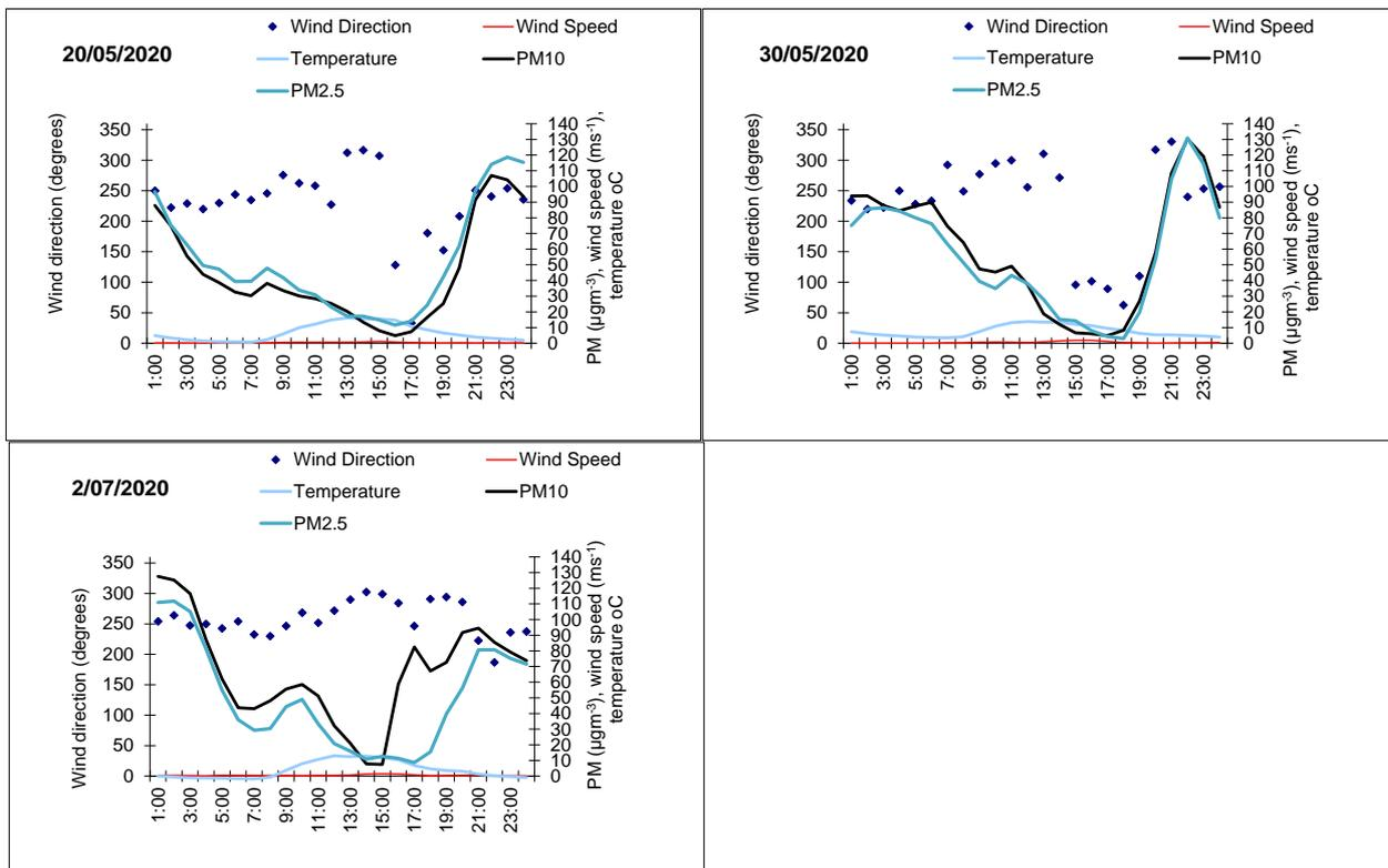
Figure 3.6: Hourly average PM<sub>10</sub>, PM<sub>2.5</sub>, wind direction and temperature on 20<sup>th</sup> and 30<sup>th</sup> May and 2 July 2020 when PM<sub>10</sub> concentrations exceeded 50 µg m<sup>-3</sup> (24 hour average).
