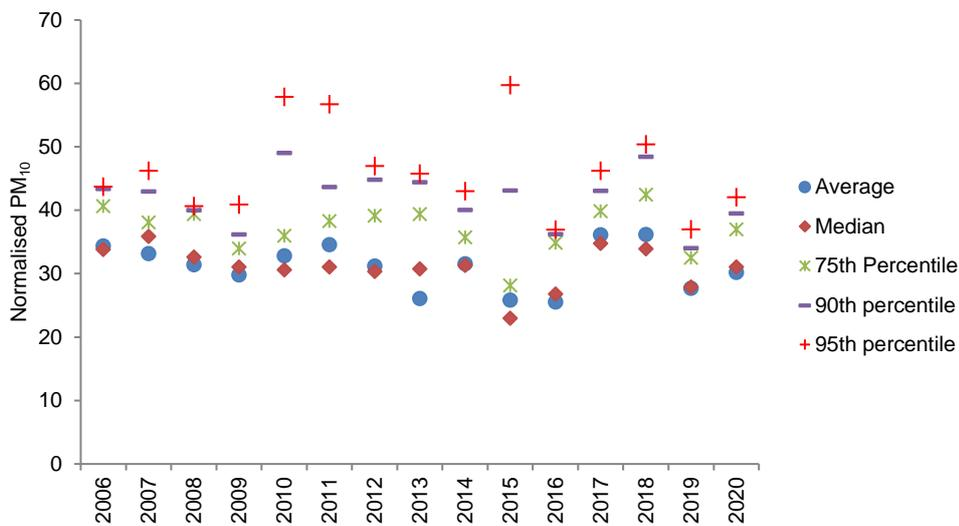
**Figure 4.1: Trends in PM<sub>10</sub> concentrations after adjusting for meteorological conditions**
