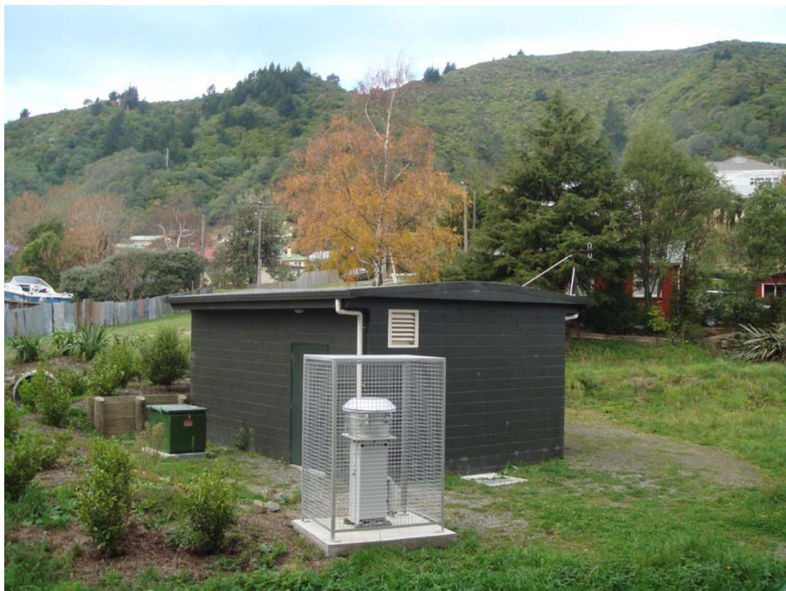
Figure 2.8: High volume sampler at the Lincoln Street site.
