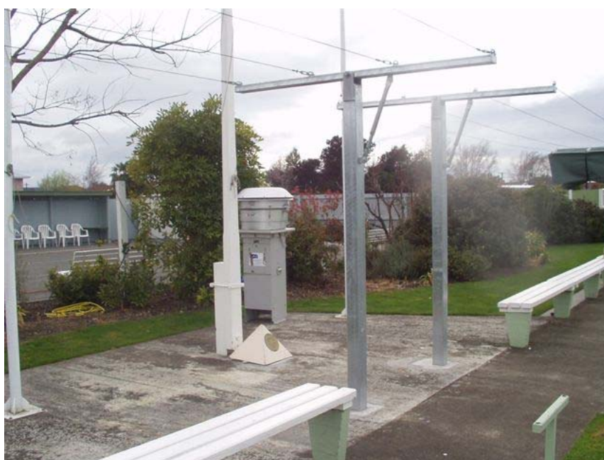
Figure 2.5: PM 10 monitor at the Redwoodtown – Bowling Club air quality monitoring site
