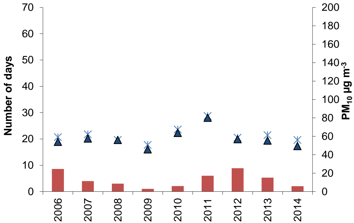
Figure 3.10: Number of days when 50 \mu\text{g m}^{-3} was exceeded, the maximum concentration and the second highest concentration from 2006 to 2014.
