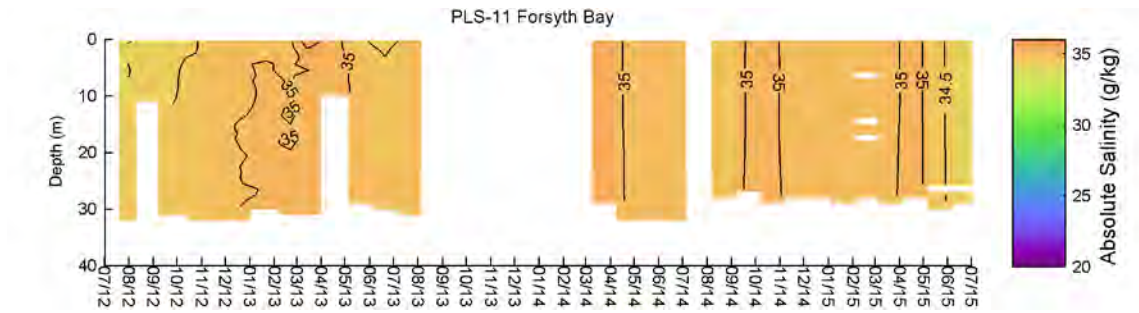
Figure 4-4: Contour plots of evolving depth profiles of salinity through time at the Pelorus stations. Data are from the monthly CTD casts. White space indicates missing/rejected data (or the maximum depth to which the cast extended).
