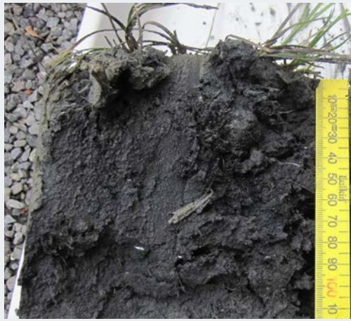
Typical sediment core at Site A showing shallow RPD layer and seagrass at the surface
