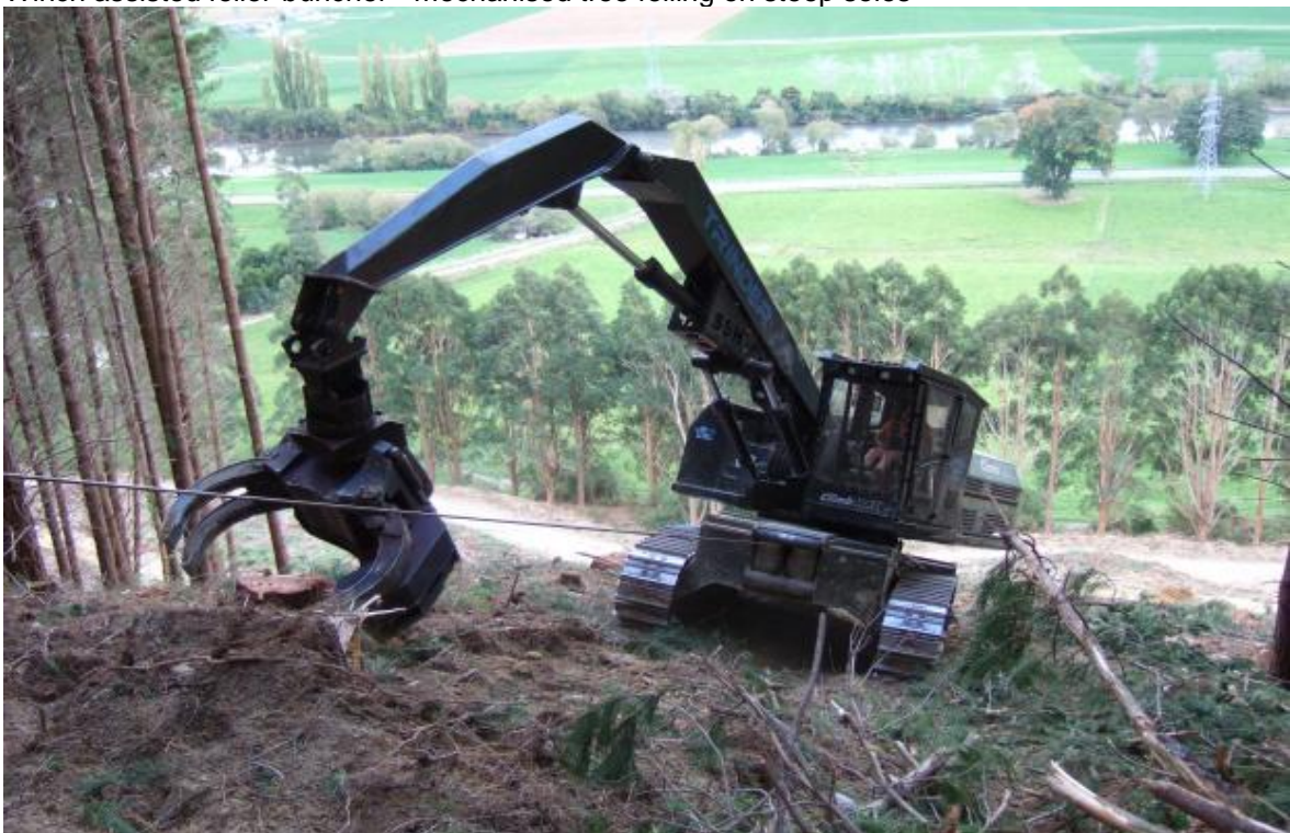
Winch assisted feller-buncher - mechanised tree felling on steep slopes
