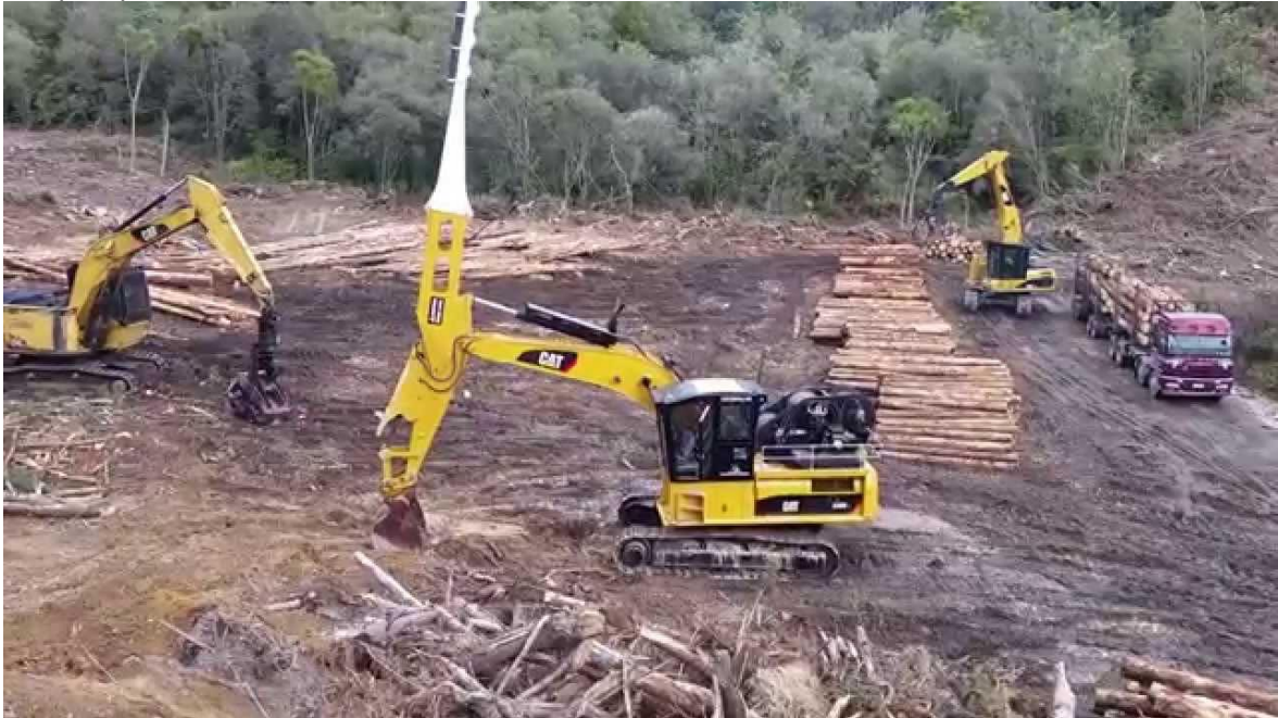
Winch assisted feller-buncher - mechanised tree felling on steep slopes
