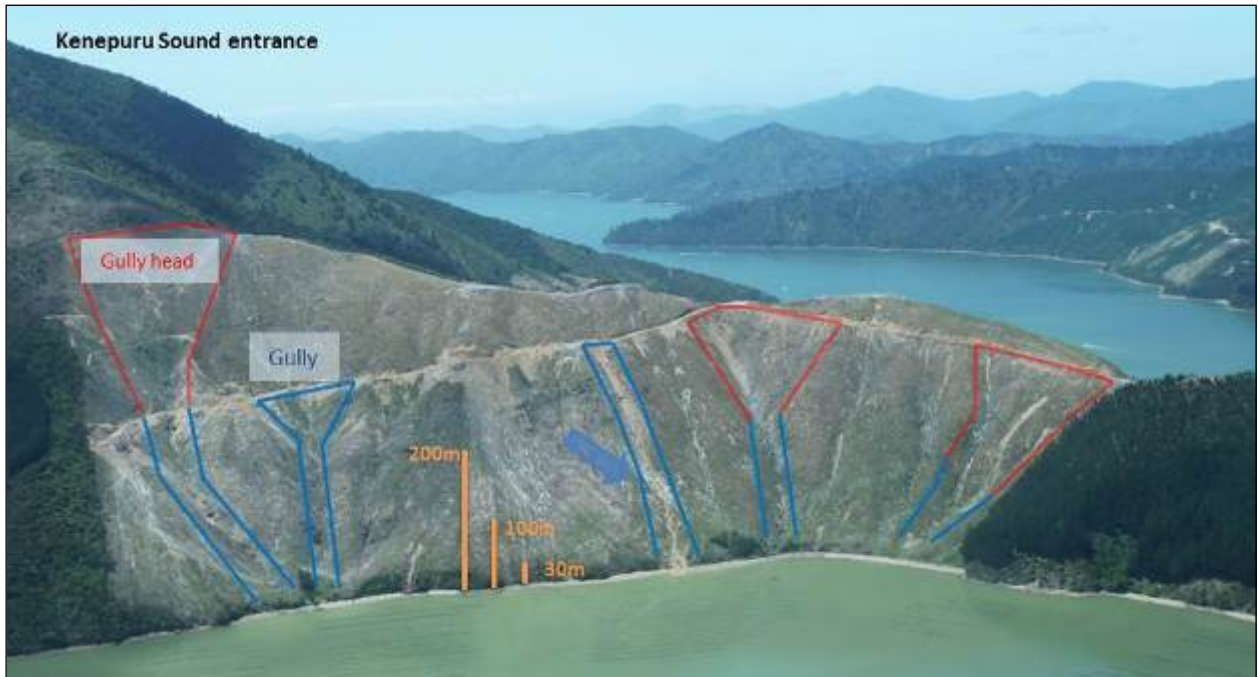
Figure A1j: Gully heads and gullies excluded from replanting; illustrative example for areas 200 metres above shoreline. This block has not been replanted since the last partial harvest in 2012 and is in pasture grass as at November 2015. Note the slip in the centre gully that occurred after harvest, shown by the blue arrow.
