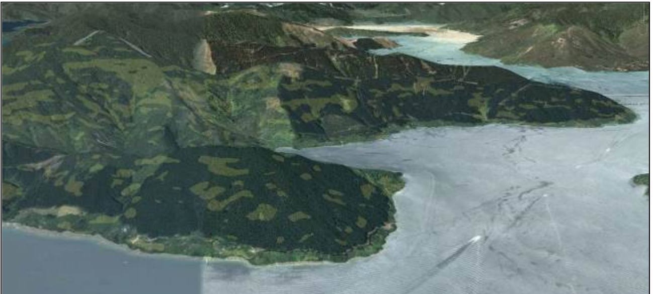
Figure 15: Digital elevation model showing modelled slopes over 35° (pale green shading) in Yncyca Bay.
