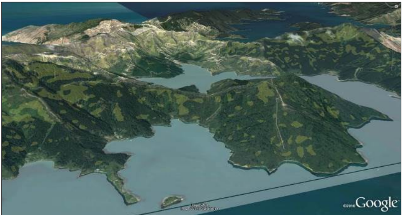
Figure 17: Digital elevation model showing modelled slopes over 35° (pale green shading) in Onepua Bay.
