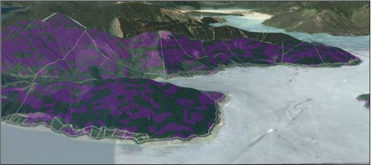
Figure 14: Digital elevation model showing modelled slopes over 30° (purple shading) in Yncyca Bay, Pelorus Sound.
