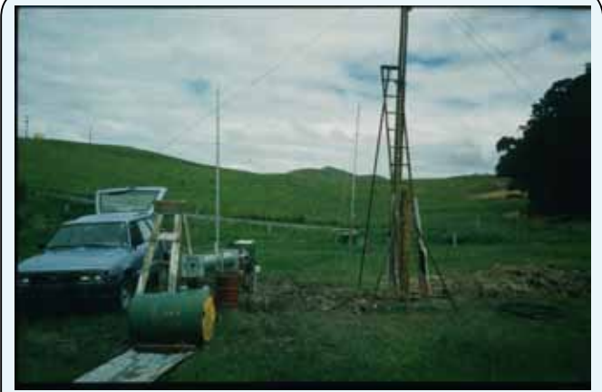
Figure 10.12: Temporary standpipe erected to measure the artesian pressures during the Benmorven Aquifer test in December 1990. The observer had to climb up the ladder and read the level of groundwater sitting in a clear plastic tube attached to the pole. This wasn't as easy as it sounds at night.
