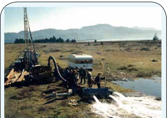
Figure 10.13: Bar test well flow measurement. Three orifice flow meters were required to measure the large flows involved with the testing of the MCRWB Bar test well (1733) tapping the high yielding coastal Wairau Aquifer in 1987.
