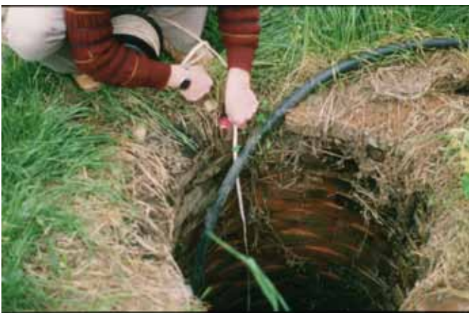
Figure 10.11: Manually measuring groundwater level in a shallow well (1856) at Benmorven in 1990
