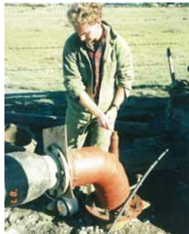
Figure 10.2: Peter Davidson manually dipping the depth to the water table during a pump test - 1987
