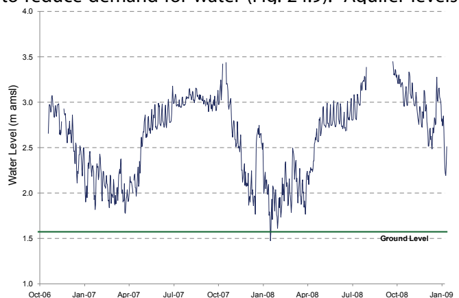
Figure 24.9: Water levels at MDC monitoring well 4402
