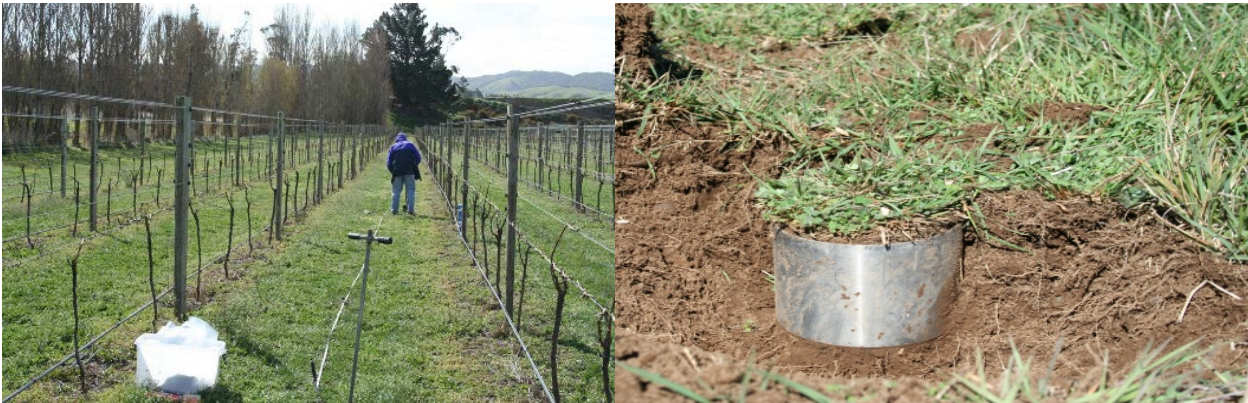
Plate 1: (a) Collecting a composite of core samples along a transect using a soil corer.
