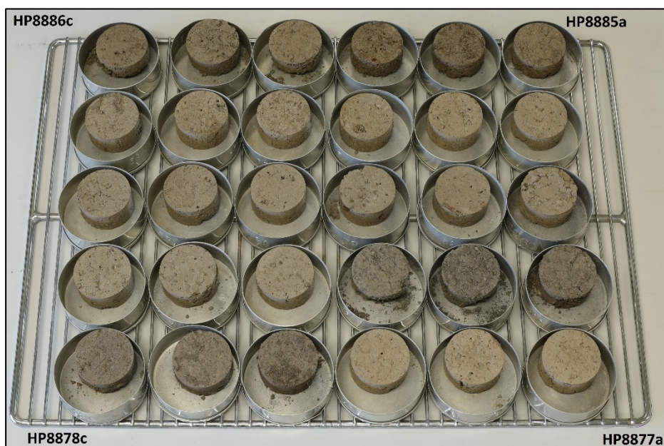
Plate 2: An example of dried cores inside their extraction rings following oven drying. Credit: D. Thornburrow, Manaaki Whenua Landcare Research
