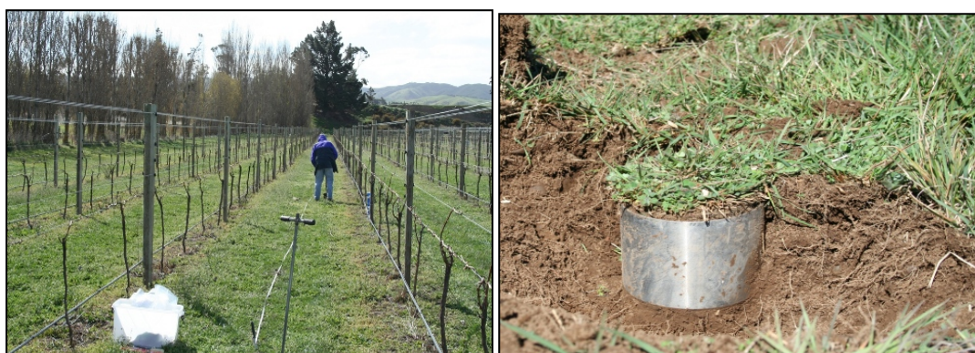
Plate 1: (a) Collecting a composite of core samples along a transect using a soil corer. (b) One of three intact core samples taken at each site, to establish the physical properties of the soil.
