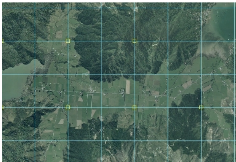
Figure 1 Map grid sheet with a 1 hectare square sample point centred on each 2 km intersection overlaying an ortho-photograph
