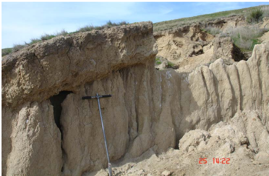
Figure 35. Expansion of erosion by the coalescence of neighbouring gullies to form a single large eroded area. The dissolution channel to the left of the auger has formed in the dispersible silty clay horizon and not in the horizon above the fragic horizon.
