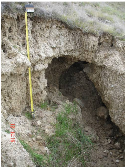
Figure 47. Tunnel gully erosion in Vernon soils. The lower layer of mixed loess and gravels found in Wither soils is absent.
