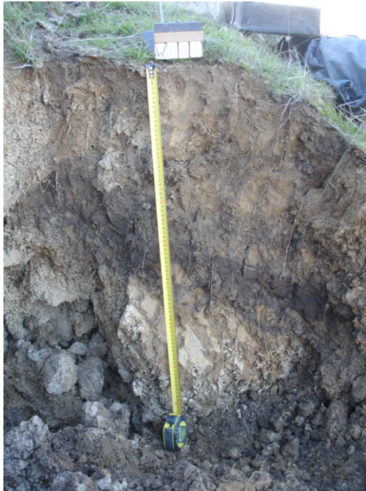
Figure 57. A soil formed on an infilled gully with a buried topsoil. An active under-runner has formed and soil collapse is occurring on the re-formed surface.
