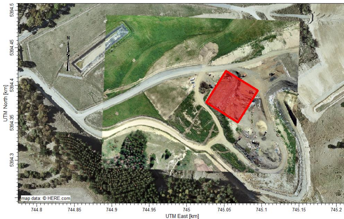
Figure 2.3: Location of active working face (assumed maximum 50 m by 50 m) at Stage 6 based on drone survey data overlaid on base map.
