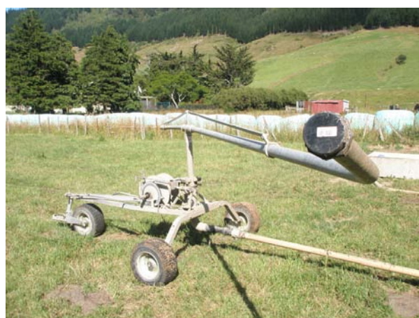
Blocking off one nozzle can increase the speed of the irrigator and minimise the discharge rate, reducing overloading
