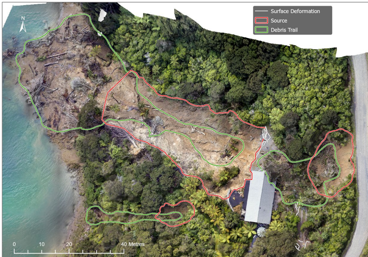
Figure 4.2 Example of landslide mapping based on RPAS imagery.
