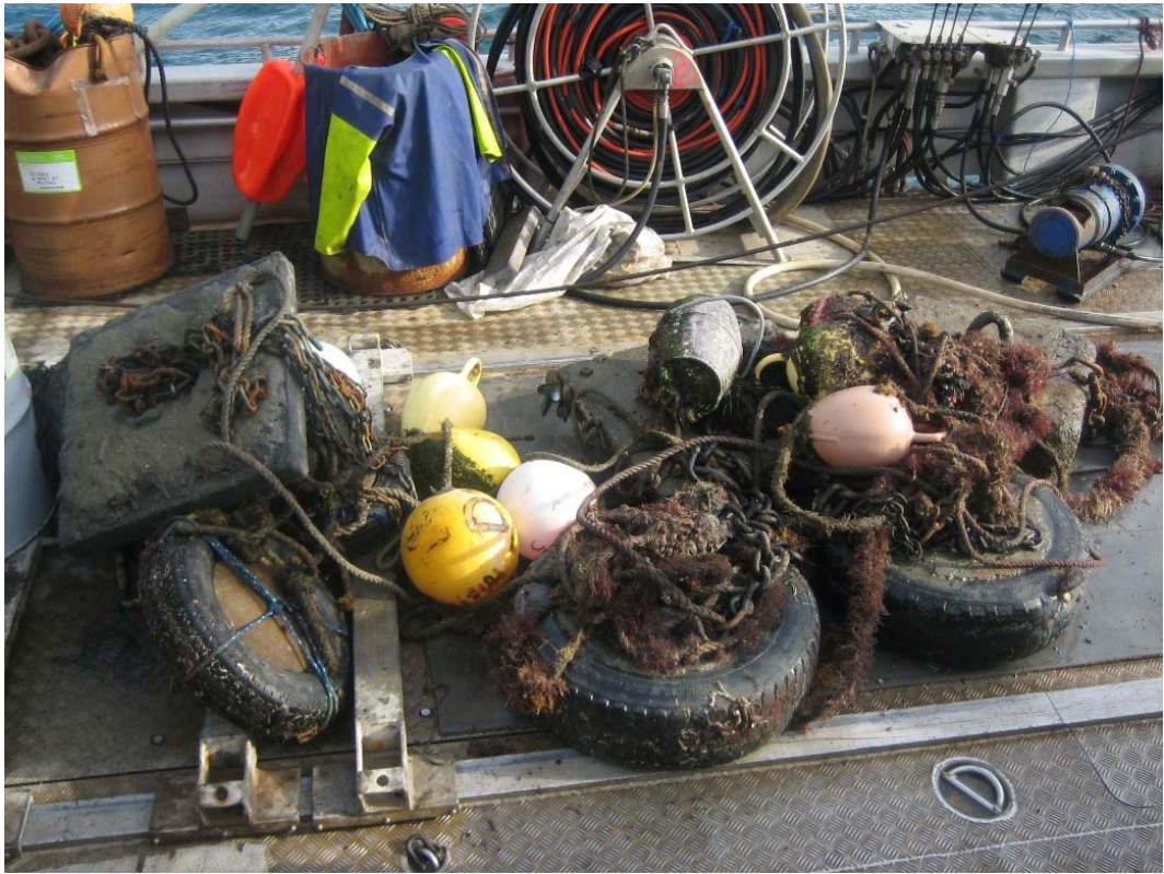
Unauthorized moorings removed from Momorangi Bay. The mooring blocks were all concrete-filled tyres.
