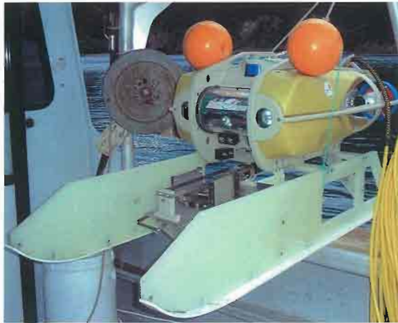
Photo 1: Remotely operated vehicle (ROV) at the surface prior to descending to the seabed. The ROV was equipped with purpose-built sediment sampler and a colour video camera and tethered to a TV/DVD recorded at the surface via an umbilical cord (right).
