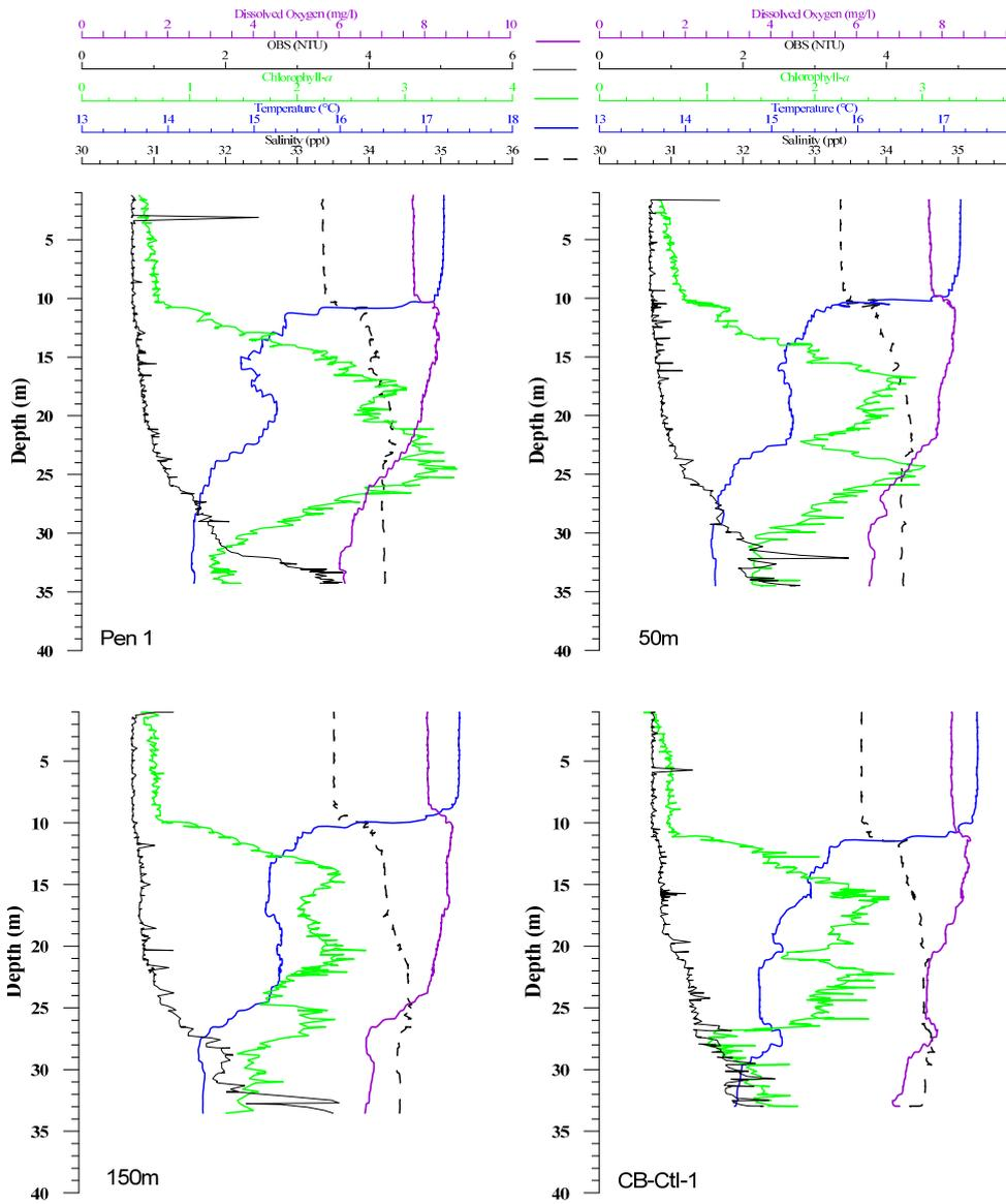
Figure 4. Dissolved oxygen, turbidity (optical backscatter), chlorophyll-a, temperature, and salinity as measured by an *in situ* sensor array raised through the water column.
