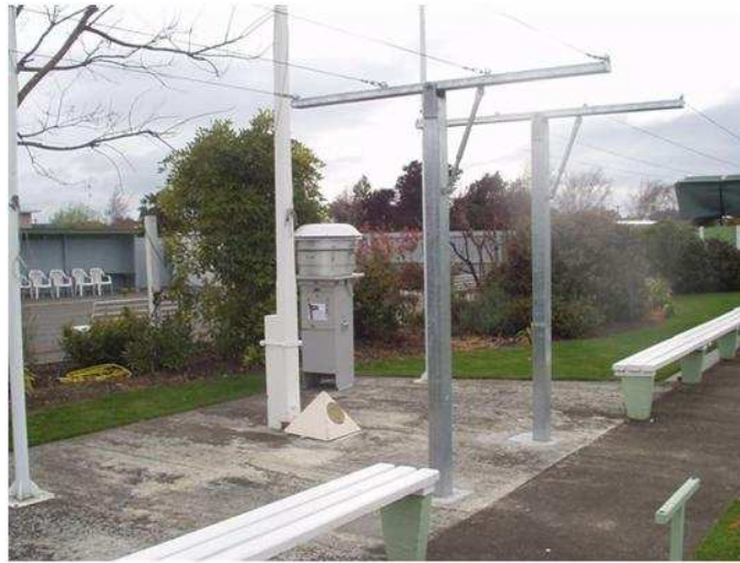
Figure 2-2: Photograph of the Redwoodtown PM 10 monitoring site with high volume sampler installed (pre-June 2006).
