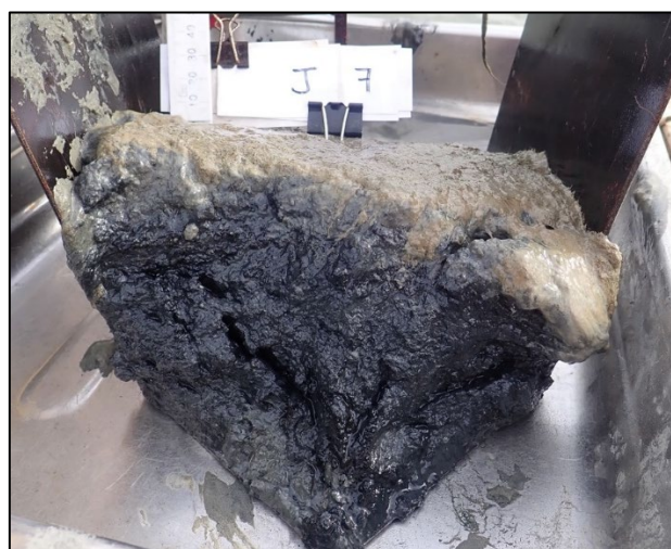
Example of colour difference between brown surface oxygenated sediments and black anoxic sediment, site J7
