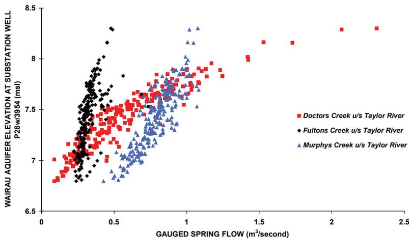
Figure 20.5: Gauged spring flow versus groundwater elevation at the substation well (3954) near the corner of Old Renwick and Murphys Roads
