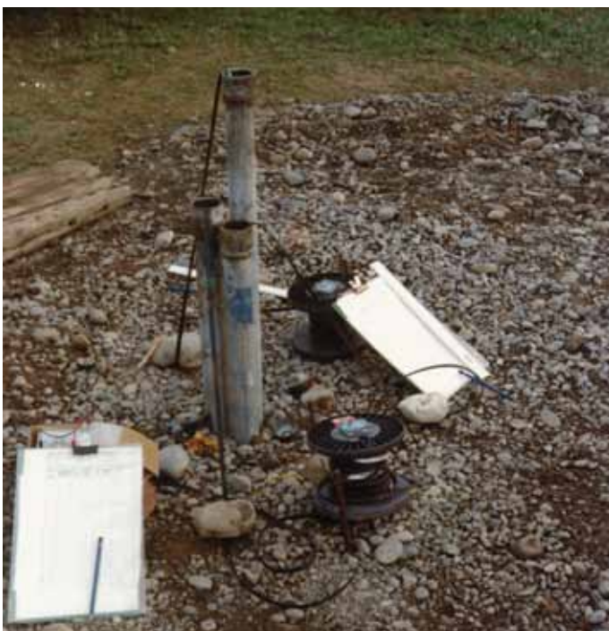
Figure 22.7: Multi-level observation well
