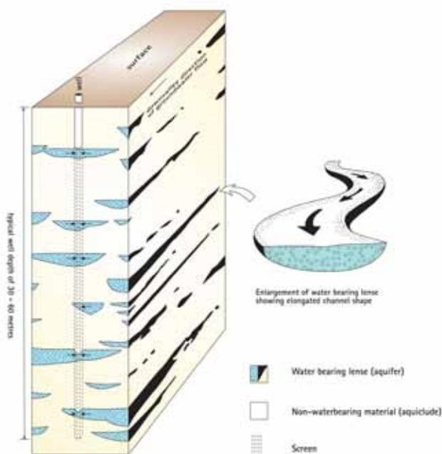
Figure 27.2: Typical Southern Valleys Aquifer structure
