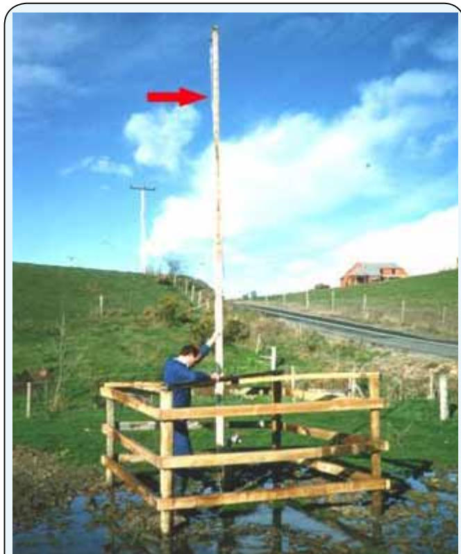
Figure 28.5: Benmorven Aquifer artesian pressure tests. The red arrow denoting the static or resting level around five metres above the general ground level
