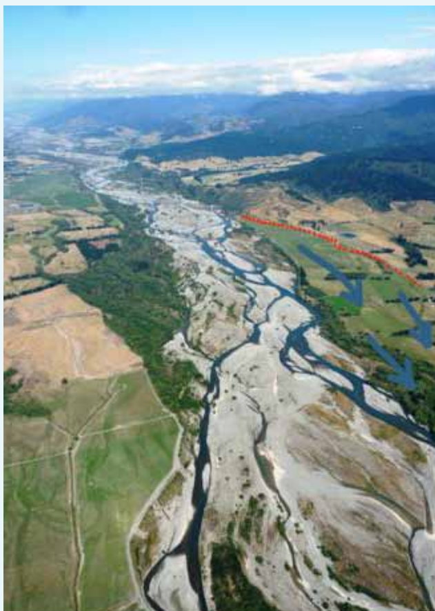
Figure 38.1: Wairau Valley looking upstream with Fabians/Bartletts Creek on the right. The dotted red line shows the location of the river terrace that separates the lower Wairau River influenced alluvial flats from the elevated terrace which is dominated by local rainfall or Fabians/Bartletts Creek flow. Arrows indicate the likely flow path of subsurface Wairau River water inferred by isotope measurements.
