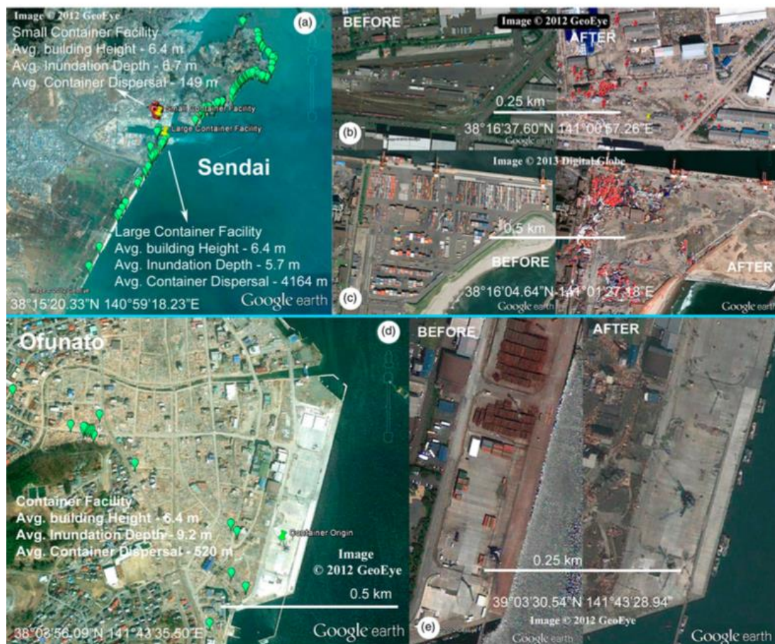
Figure 12. Looking at container dispersal from container storage facilities following the 2011 Tohoku tsunami. (a) Sendai region and port. (b) Small container facility at Sendai port before and after the tsunami. (c) Large container facility at Sendai Port before and after the tsunami. (d) Ofunato region and port. (e) Ofunato container facility before and after the tsunami. Source (Naito et al. 2014).
