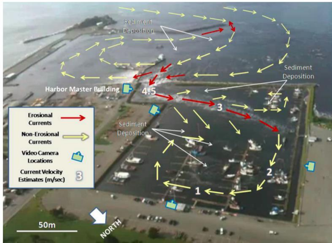
Figure 16. Tsunami in-flow regime map for Crescent City Harbor showing the maximum observed tsunami current velocity values over the span of the first 3.5h of the 2011 Tohoku tsunami. Numbers show estimated surface velocities (m/s), and arrows indicate flow direction based on 14 ground-level and aerial videos taken of the event. Source (Admire et al. 2014).
