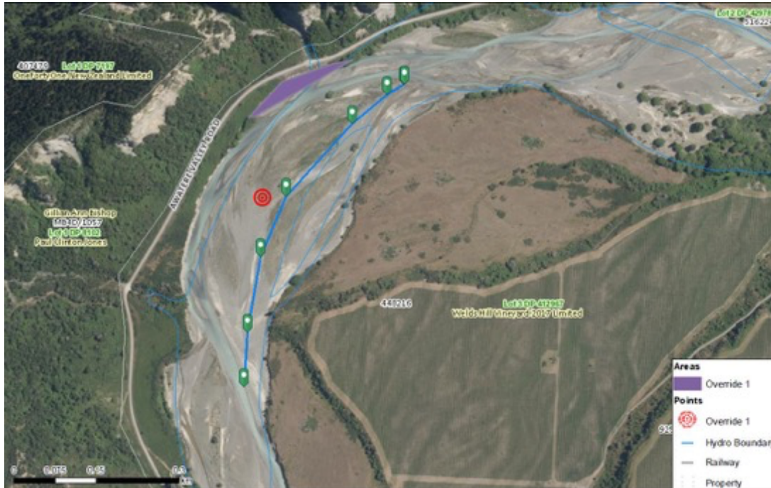
Above: Medway Road - Jordan River. The river is undercutting into the bank on the left (shown in purple) to the marked blue channel further to the right.
