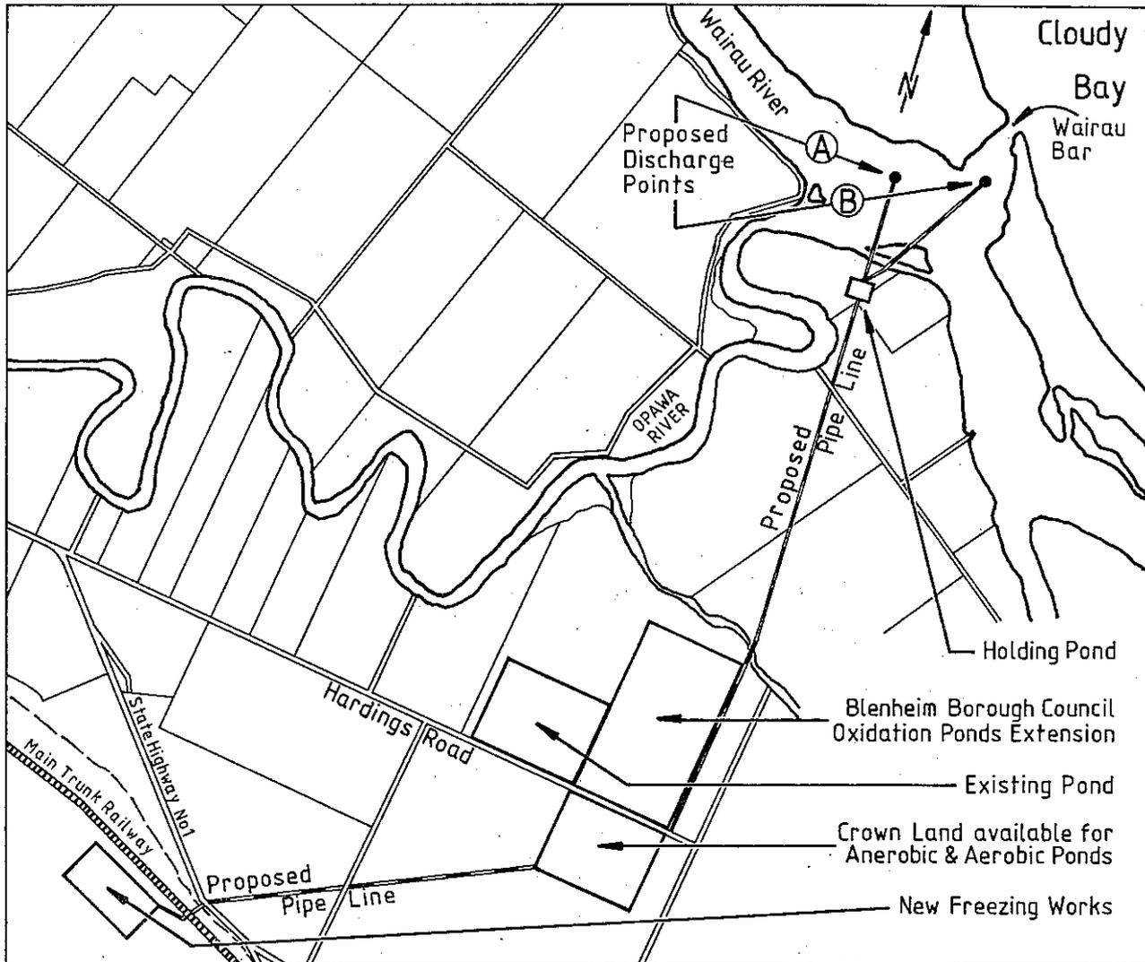
Fig. 1.2. Plan showing the freezing works site, the proposed sites of the aerobic and anaerobic ponds, the proposed route of the pipeline and alternative discharge points.
