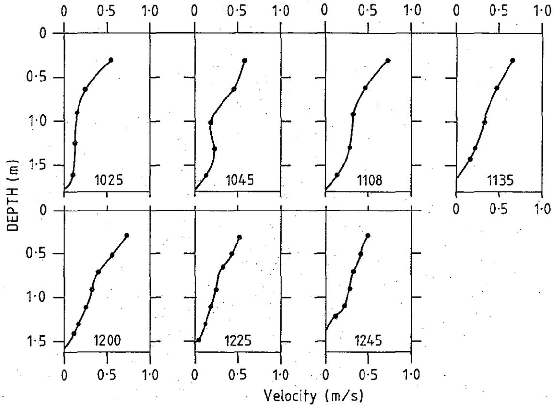
Fig. 7.1. Ebb tide velocity measurements taken on 6.4.81 at Site A (see Fig. 1.2.). High tide 0748 hr (+0.52 m), low tide 1411 hr (-0.42 m). Flow at Tuamarina 20 cumecs (approximately). (Modified from Hume and Williams, 1981, Fig. 5A).
