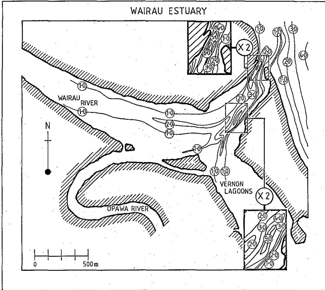
Fig. 6.1. Bathymetric map of the Wairau River Estuary and Wairau Bar (based on the map prepared by the Marlborough Catchment Board in association with the Marlborough Harbour Board and the Department of Lands and Survey).
