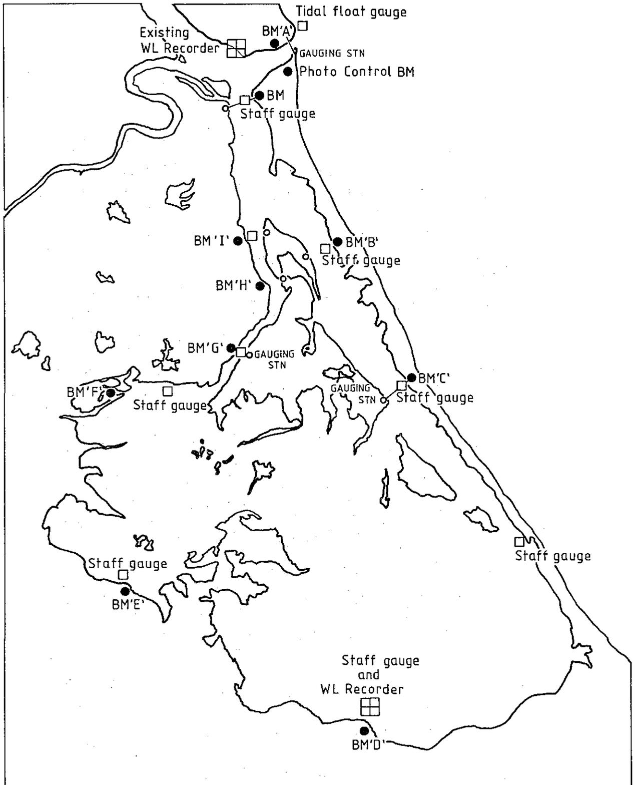
Fig. 7.3. Positions of the gauging stations from which the data for Fig. 7.4 was obtained.
