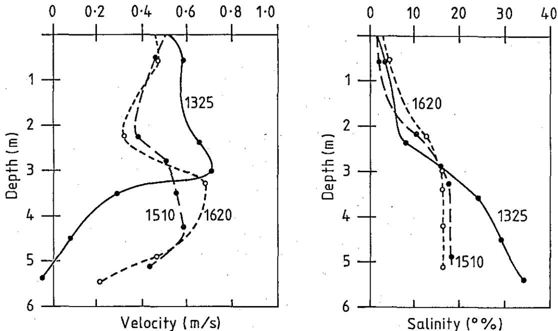
Fig. 7.2. Ebb tide velocity and salinity profile measurements taken on 22.6.81 at Site B (see Fig. 1.2). High tide 1005 hr (+0.53 m), low tide 1630 hr (-0.88 m). Flow at Tuamarina 90 cumecs (approximately). (Modified from Hume and Williams, 1981, Fig. 5B).
