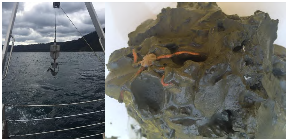
Figure 1-30: Dietz-Lafond grab used for sediment sampling (left) and sample on collection plate (right).
