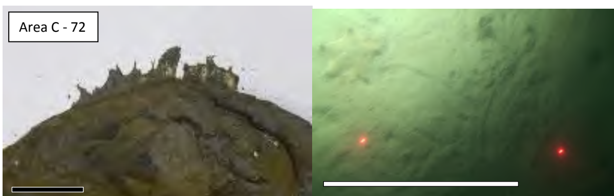
Site C72 physical sample (left), scale = 5 cm; and seafloor image (right), scale = 20 cm.
