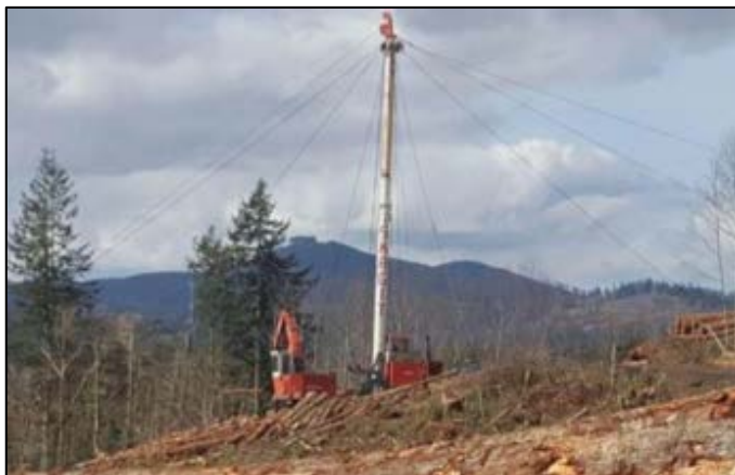
Figure 9: (L) Large tower hauler, suitable for large settings and long haul distances on steep terrain (photo: SCION). (R) Forest harvested predominantly by hauler, Yncyca Bay, Pelorus Sound/Te Hoiere, June 2016.
