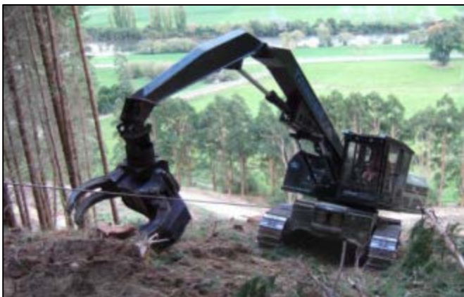
Figure 10: (L) Winch assisted feller-buncher – mechanised tree felling on steep terrain (photo: SCION). (R) Forest harvested by ground-based machines, Mud Bay, Pelorus Sound/Te Hoiere, November 2016.
