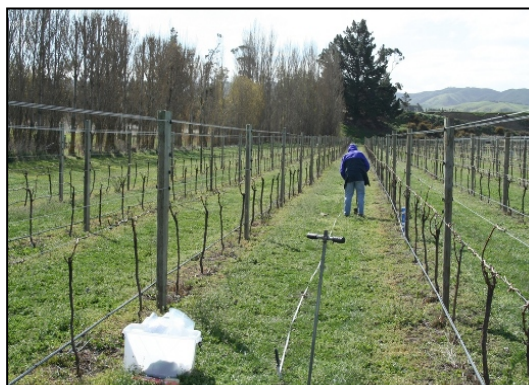
Plate 1 (a) Collecting a composite of core samples along a transect using a soil corer. (b) One of three intact core samples taken at each site, to establish the physical properties of the soil.
