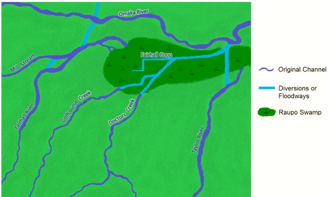
Figure 18: Original stream channels and stream diversions in the lower Doctors Creek catchment [32].
