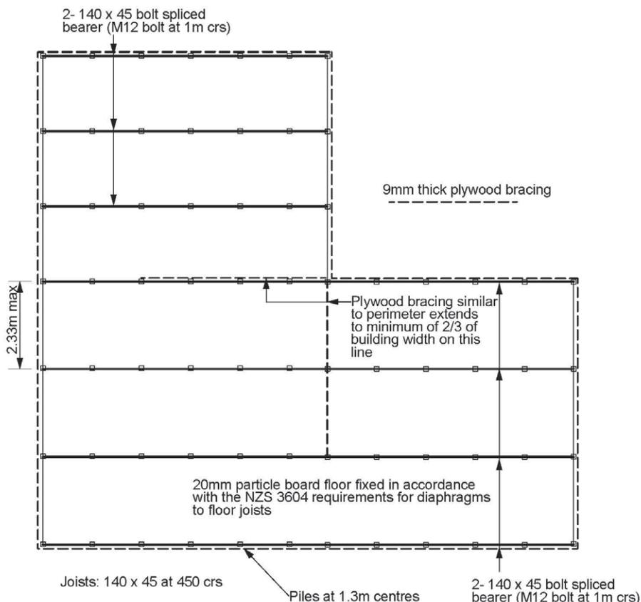
Figure 15.16: Perimeter foundation details for Type 1 surface structure
