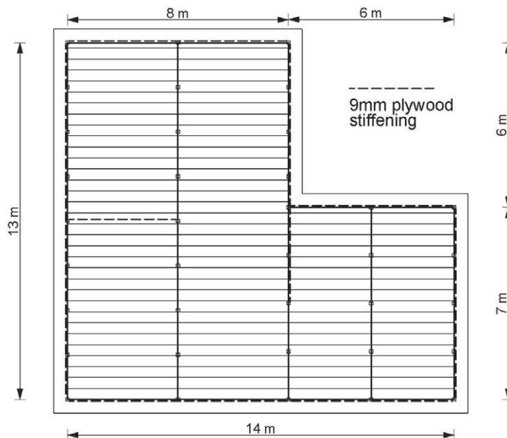
Figure 15.18: Section through Type 2A surface structure at the timber piles
