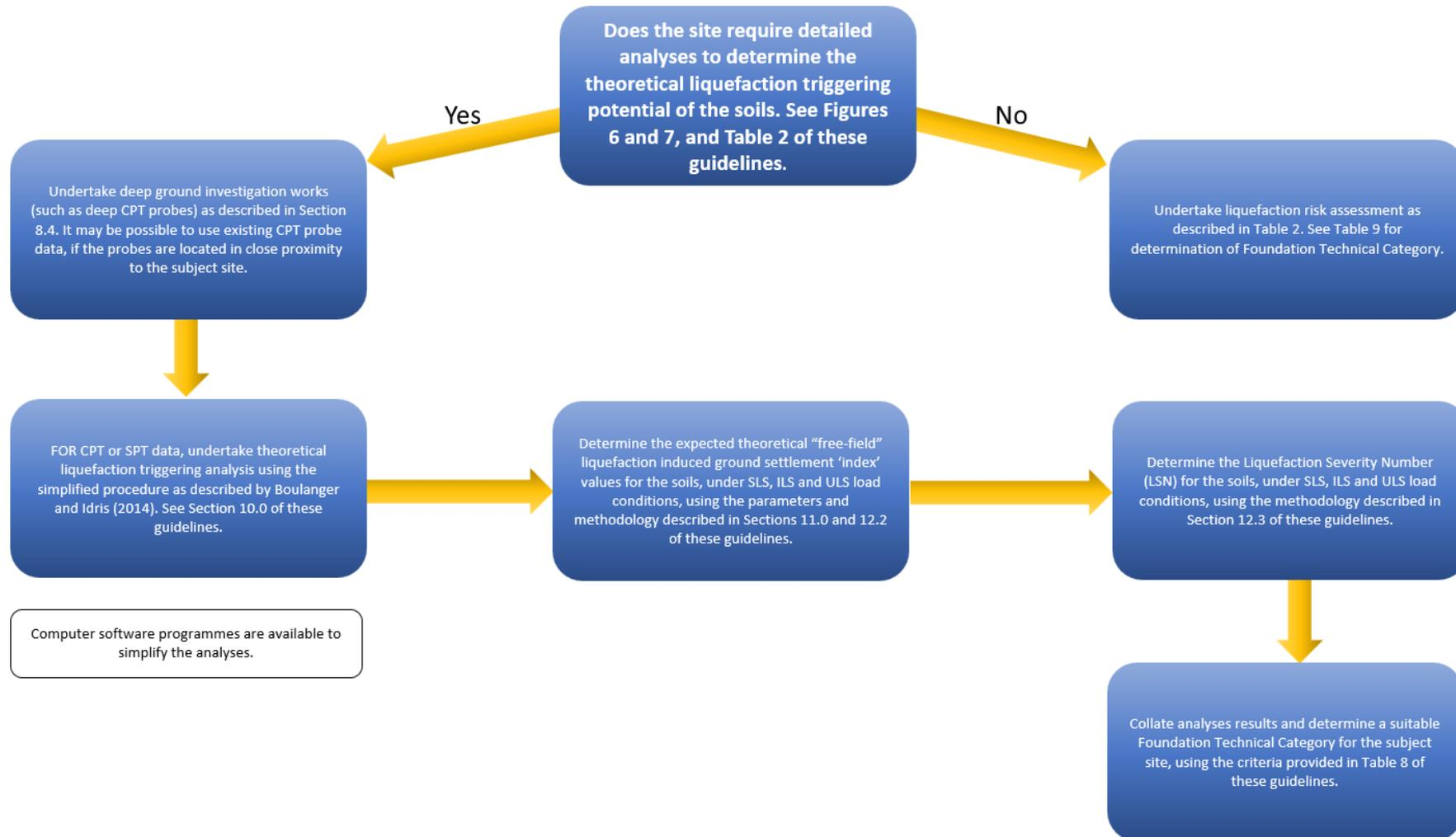
**Figure 9** *Flowchart, Determination of theoretical liquefaction potential characteristics.*
