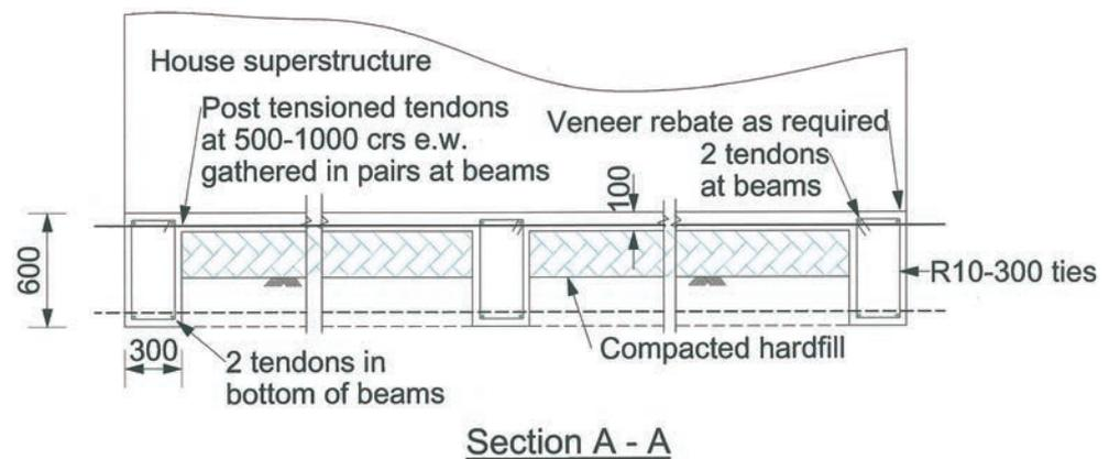
Note: Post tensioning strands are either 12.9 mm or 15.2 mm diameter and factory coated with grease inside an HDPE sheath, giving an overall outside diameter of 17 to 20 mm respectively. Strands are tensioned to provide 0.5-1.0 MPa compressive stress in the concrete.
