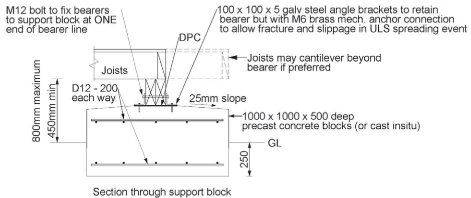
**Type 3B – Steel beams over prestressed concrete beams (stiff platform)**
