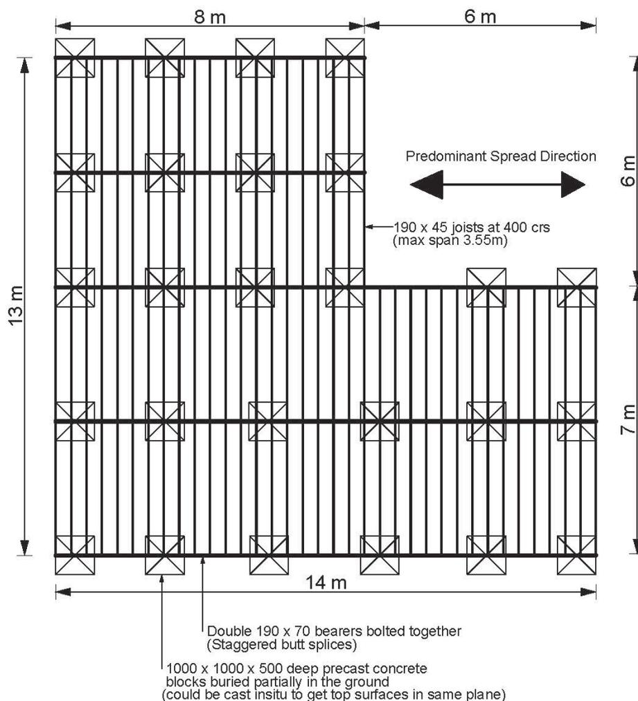
**Figure 15.23: Type 3A surface structure - Detail at supporting blocks**
