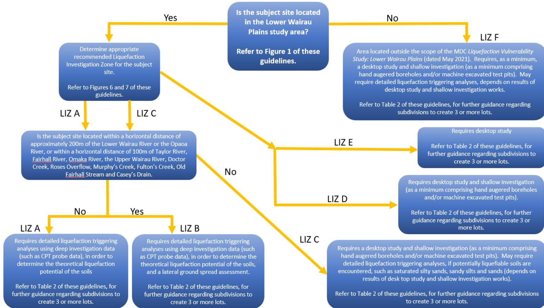
**Figure 8** Flowchart: Determination of suitable geotechnical investigations for liquefaction potential assessment purposes (general).
