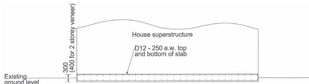
Note: NZS ground clearances adjacent to house foundation must be complied with. DPC omitted for clarity.
