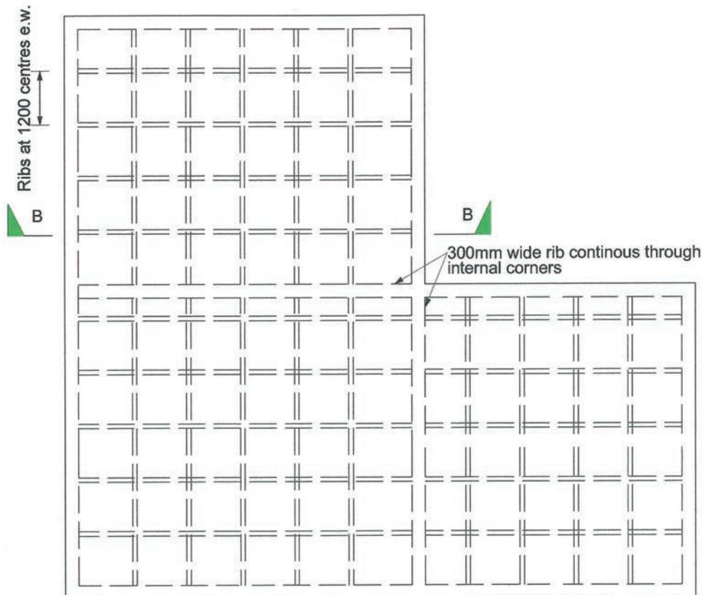
Note: Reinforcing details are not sufficient for two-storey heavy-weight cladding (brick veneer) with either a heavy or light roof.
