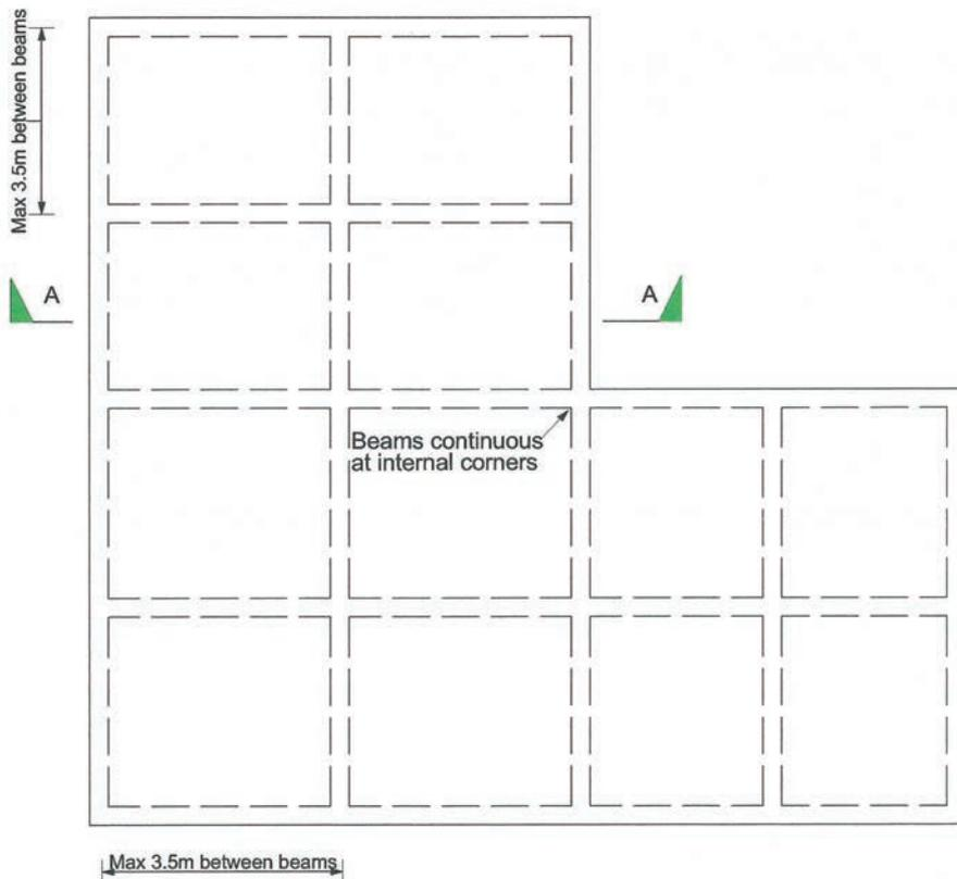
Note: Reinforcing details are not sufficient for two-storey heavy-weight cladding (brick veneer) with a heavy roof but can be used for a two-storey heavy-weight cladding with a light-weight roof.
