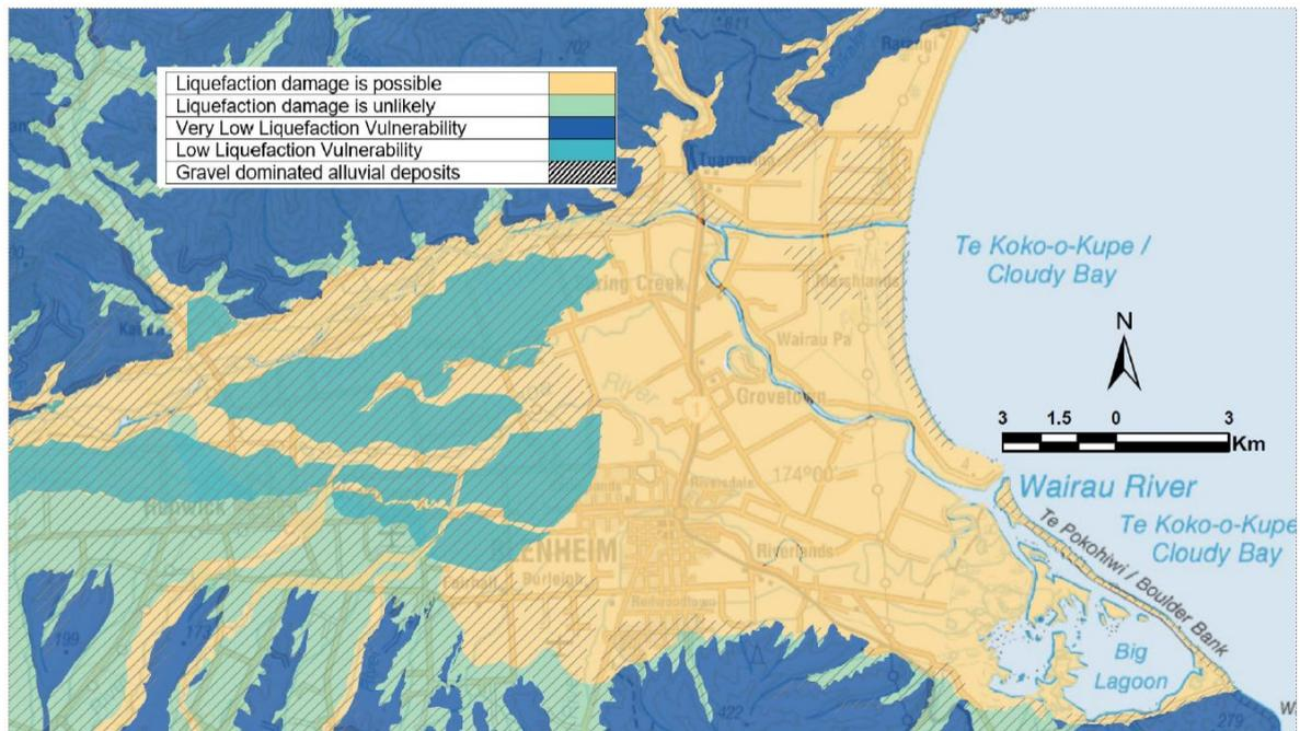
**Figure 5** Summary of liquefaction vulnerability category map for the Lower Wairau Plains and base of gravel greater than 5 m<sup>5</sup>.
