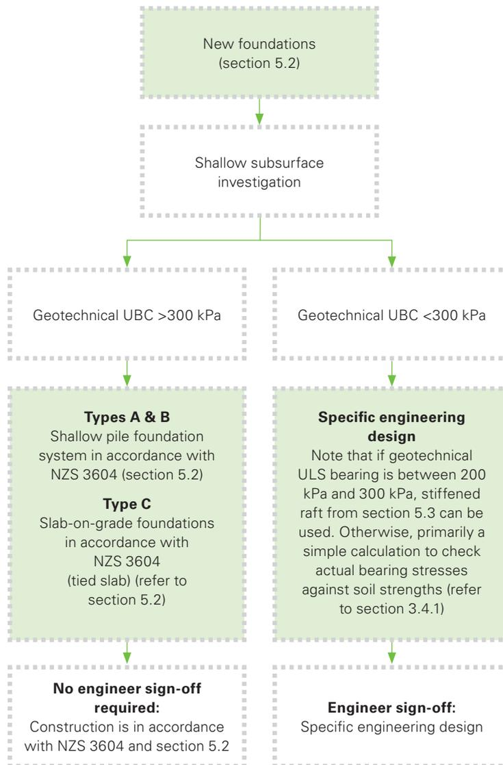
Figure 5.2: Overview of process for new foundations on TC2 sites
