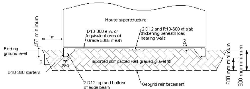
**Option 2** – Construct a thick slab foundation over the existing soil.
