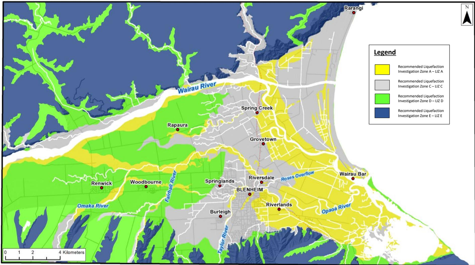
**Figure 6** Liquefaction Investigation Zones (LIZ) for the Lower Wairau Plains – Overall Plan.
