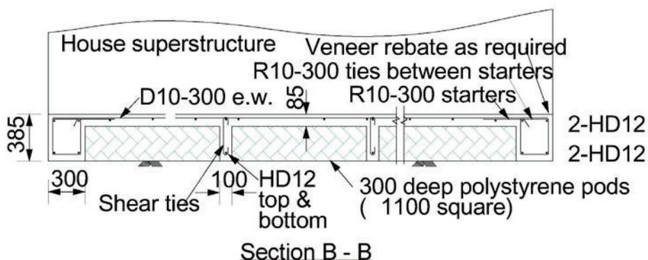
The ground immediately beneath the polystyrene and ribs must have a minimum geotechnical ultimate bearing strength of 200 kPa, or the system should be subject to specific engineering design (refer to section 3.4.1). Shear ties in accordance with NZS 3101 are required in the ribs.
