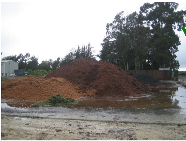
Grape Marc and Leachate Contained on Concrete Pad. Leachate runs off to Wastewater System
