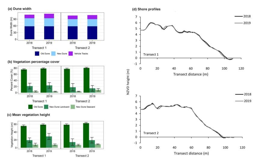
**Fig. 4.6** Preliminary results from beach monitoring at Long Point over the summers of 2018 and 2019. (a) dune width, (b) percentage cover, (c) mean vegetation height, (d) shore profiles. The new dune zone is defined as the vegetation seaward of the estimated position of the old (pre-earthquake) dune toe, and is split in half (new dune landward and seaward) in graphs (b) and (c). Error bars are standard error of the mean for 2 x 2 m plots surveyed within each area.
