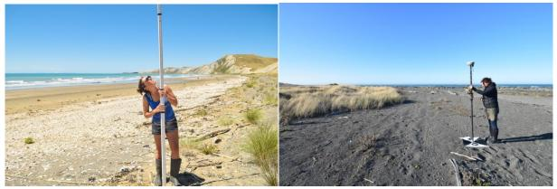
**Fig. 3.2** Beach response monitoring. (a) Beach monitoring transect at Mussel Point. (b) RTK-GPS survey underway at Airstrip Beach to support UAV (drone) mapping of the uplifted beach.
