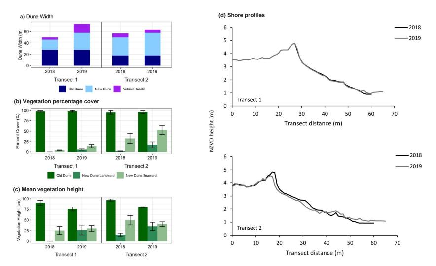
**Fig. 4.9** Preliminary results from beach monitoring at Aerial Beach over the summers of 2018 and 2019. (a) dune width, (b) percentage cover, (c) mean vegetation height, (d) shore profiles. The new dune zone is defined as the vegetation seaward of the estimated position of the old (pre-earthquake) dune toe, and is split in half (new dune landward and seaward) in graphs (b) and (c). Error bars are standard error of the mean for 2 x 2 m plots surveyed within each area.
