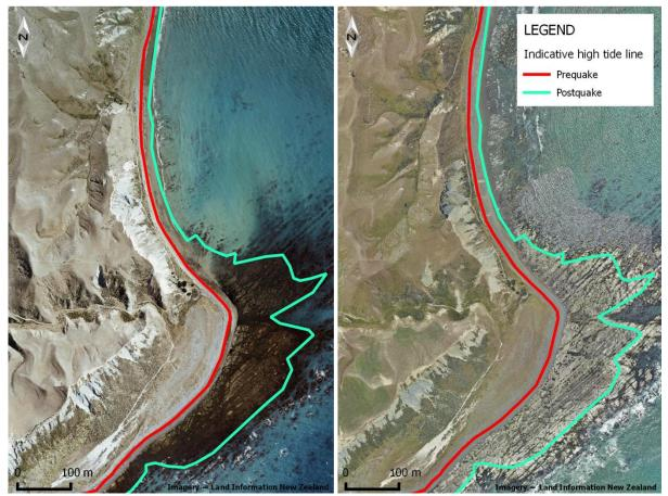
**Fig. 1.1** Example of shoreline position changes associated with tectonic uplift at Long Point on the Marlborough coast showing pre-quake imagery (left), and post-quake imagery (right).
