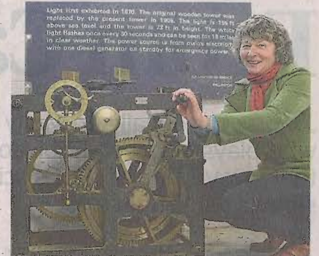
Sally Peter winds the crank of the clock mechanism that rotated the light beacon of Cape Campbell lighthouse.
