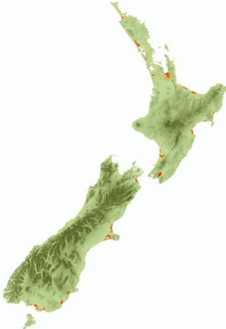
Figure A4.9: Indicative areas that will require risk analysis to establish their likely vulnerability to coastal inundation as a result of sea-level rise – either directly (e.g., inundation during storm events) or by the impact of sea-level rise on the drainage of low-lying coastal lands. The shaded red and orange areas show approximate land levels less than 5 m and 10 m above sea level, respectively: they have been extracted from reprocessed topography data collected by the Space Shuttle Radar Topography Mission (NASA). Accuracy of the topography is around 5–8 m (Ministry for the Environment)
