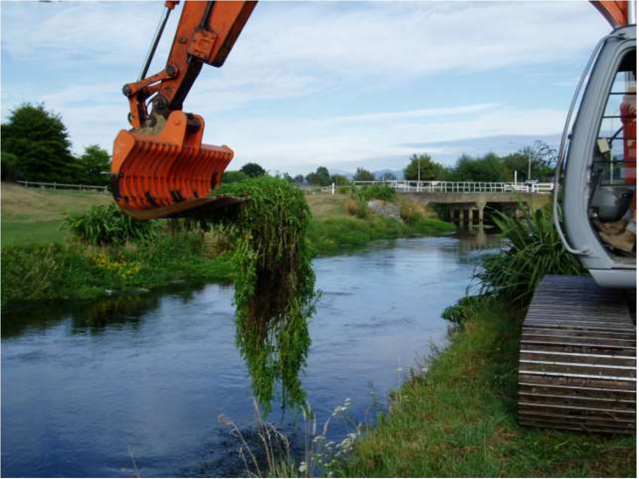
Photo 1 - Tinned bucket that allows eels and other life to fall back into the river.
