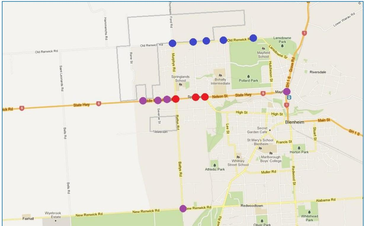
The close proximity of these intersections to each other means that if one intersection has been improved there could be a shift in traffic flow so that the adjacent intersection improvements could be deferred. Furthermore the signalisation of a single intersection can often alleviate intersection delays downstream of the traffic signals as the platooning effect of green and red waves often provides gaps in flow for vehicles to enter from the side roads.
