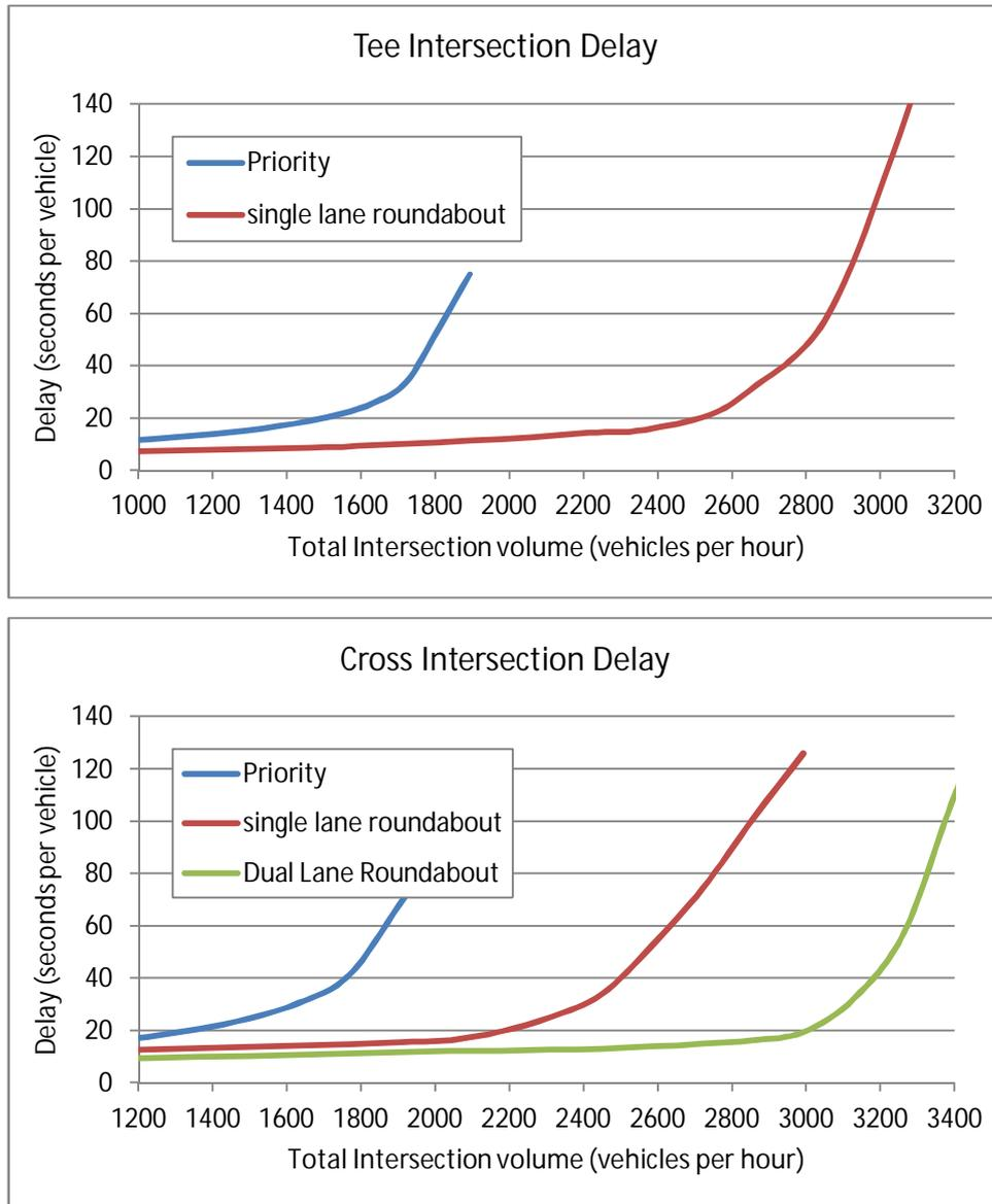
Table 12 provides the approximate intersection flow when Level of Service E is reached and when an intersection will require assessing to undertake improvements to reduce congestion back to a more acceptable level such as Level of Service C.
