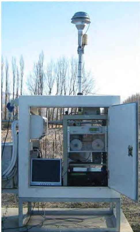
Photo 5 – example of the NO 2 /SO 2 monitoring equipment and housing.
