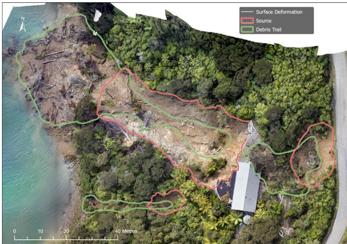
Figure 4: Example of landslide mapping based on drone imagery.
