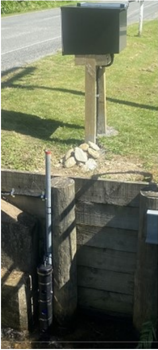
Figure 1: The new dissolved oxygen sensor in the Marlborough Sounds Freshwater Management Unit and a graph showing recent measurements over the course of two days.
