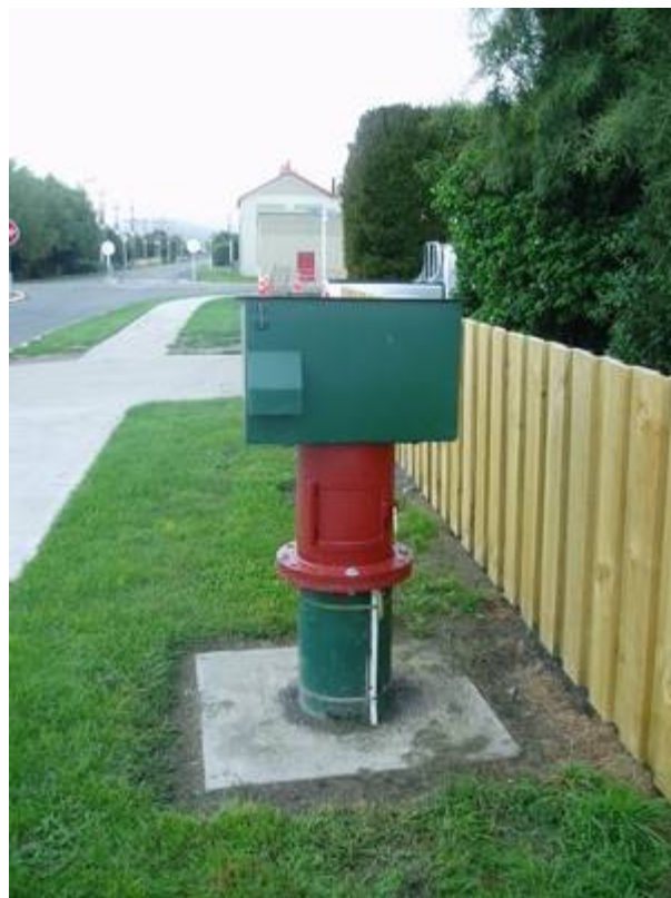
Photograph showing MDC Murphys Road monitoring well P28w/3954 looking north towards Old Renwick Road intersection with well in foreground and instrument housing on top.
