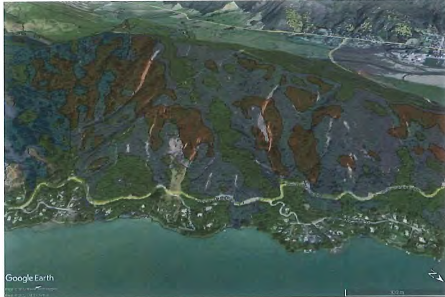
Figure 3. The area between Belvue Bay Road and Moenui Road showing multiple landslide scars after the July 2021 rainfall event. The coloured shading shows slopes: <26 degrees (green), 26-35 degrees (pale) and >35 degrees (red). Using the low (green) ESC to determine resource consent status may result in serious errors.
