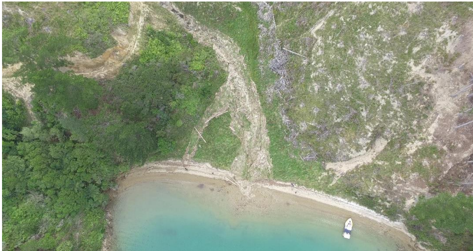
Figure 6. Commercial forest on land in Port Underwood with a significant mid-slope area >35 degrees after Cyclone Gita 2018. Note the debris flows in the gullies and significant “scalping” of topsoil along extraction paths. The two images cover the top of the catchment to the shoreline.
