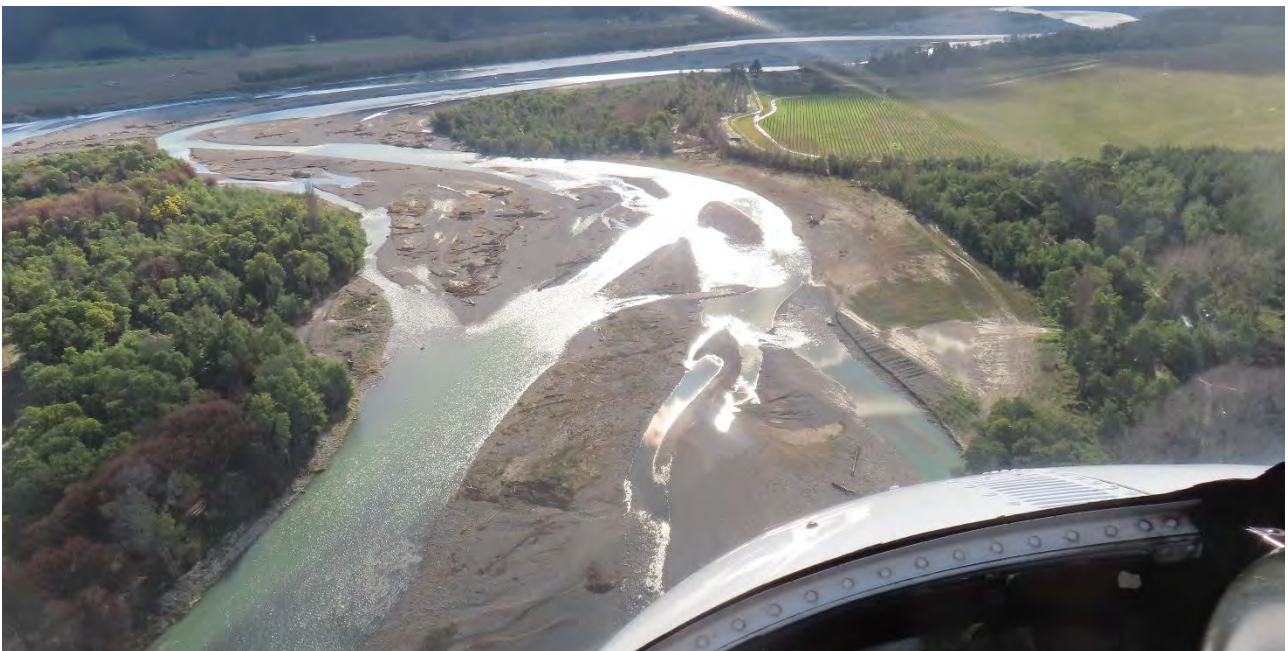
Figure 6: Looking downstream, Waihopai River upstream of the confluence during the June 2026 event, showing the active channel established against the true right bank and increasing the risk to stopbank integrity in a subsequent flood event. The remains of the temporary gravel bund installed to protect the stopbank are visible in the bottom right.
